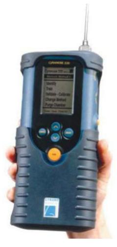
in the on-board database for easy access and reporting. Rapid qualitative measurements or "sniff" tests lasting 5 to 15 seconds for discrimination and identification can be extended to quantitative headspace analyses using suitable standards for calibration.
